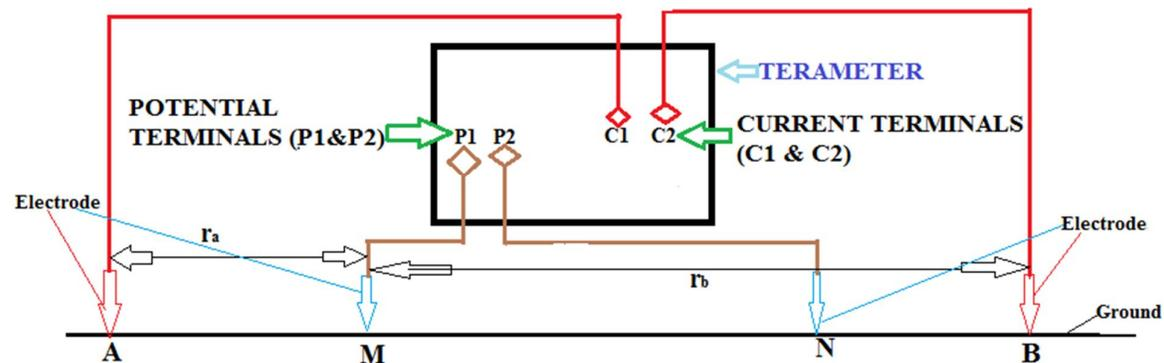
Figure 2: Schematic representation of four electrode arrangement in the Schlumberger array as connected to terrameter.
