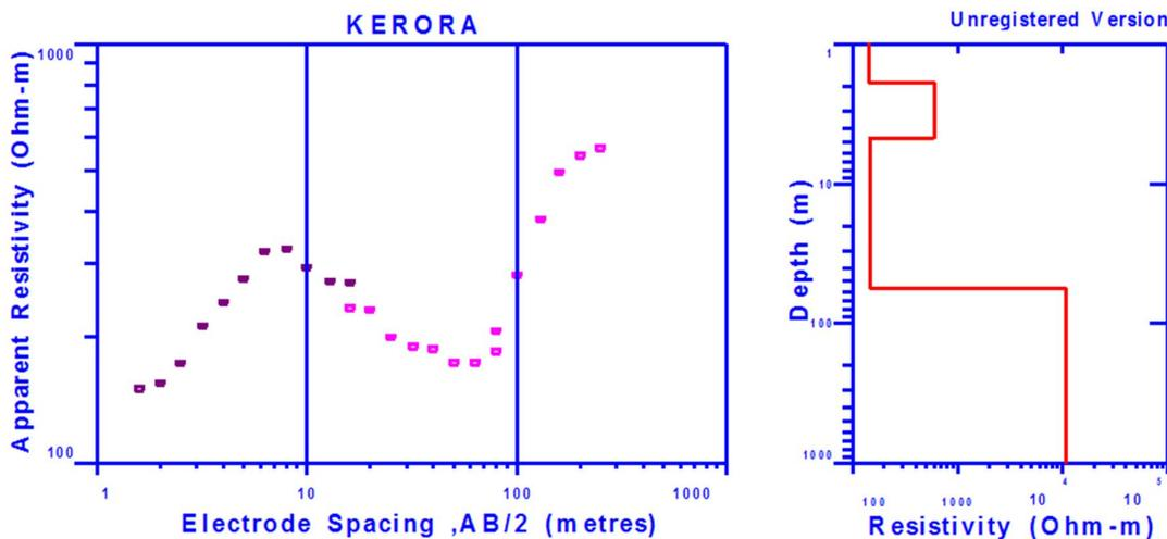
Figure 5: A curve showing the variation of apparent resistivity with electrode spacing AB/2, which represents the depth of investigation and model interpretation showing the depth, thickness and resistivity of each layer at VES 3.
