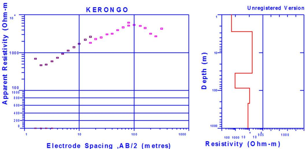
**Figure 4: A curve showing the variation of apparent resistivity with electrode spacing AB/2, which represents the depth of investigation and model interpretation showing the depth, thickness and resistivity of each layer at VES 2**
