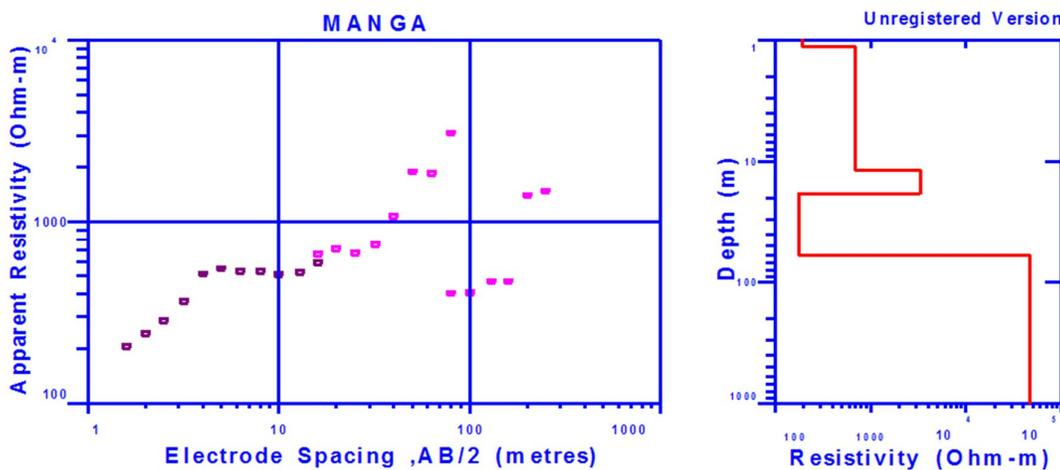
Figure 6: A curve showing the variation of apparent resistivity with electrode spacing AB/2, which represents the depth of investigation and model interpretation showing the depth, thickness and resistivity of each layer at VES 4
