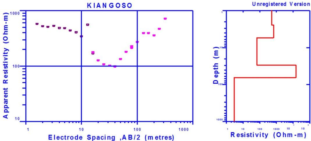
**Figure 3: A curve showing the variation of apparent resistivity with electrode spacing AB/2, which represents the depth of investigation and model interpretation showing the depth, thickness and resistivity of each layer at VES 1**
